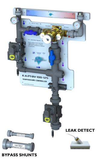
Provided in event of an electrical valve failure. Simply un-screw union nuts on electric valve and replace with bypass shunt until repairs are complete.
