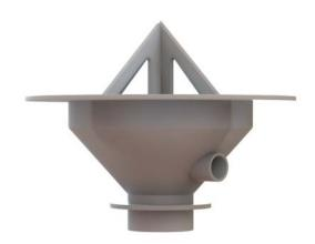
**Mechanics:** Suction is applied to the media loader via a 5hp or greater vacuum cleaner. The media bag is punctured by the gusset on top of the loader and the media is drawn down into the tank.
